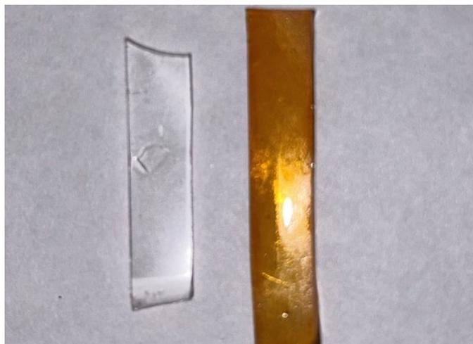
**Figure 2.** Photograph of 75 mol% phenyl silicone elastomer, unexposed and after 6.2 MGy of gamma radiation in air. The change in color is likely due to oxidation.
