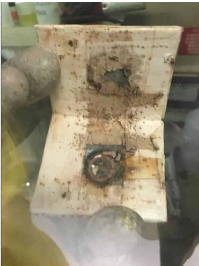
**Figure 1.** Sample of lead contained Pa-231, legacy material at SRNL.
