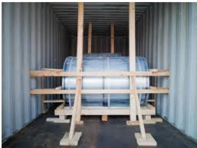
**Figure 1.** Scaffolding holding in place a container containing low level waste items within a shipping cargo container.
