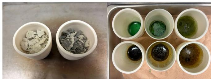
Figure 2. Carbon-containing ECMs and non-Carbon ECMs prior to remelt (left) and after remelting at various temperatures (right)
