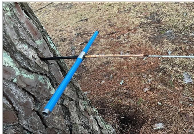
**Figure 4.** Bore wood core collection from a pine tree. Radial pattern (light/dark) within the core indicates annual increment growth. Hg concentration can be determined on each year (one ring), averaged though years, or as several years analyzed together (several rings). Analysis of Hg isotopes may require combining rings (spanning several years) to meet quality control requirements of the MC-ICP-MS instrument.
