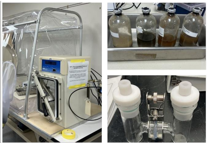
**Figure 2.** Testing Setup for Landfill Leachate. Left, Anaerobic Coy chamber for anoxic manipulations of microbes. Top right, Incubations of Landfill leachate with granular activated charcoal. Bottom right, electrolysis cell for future testing.
