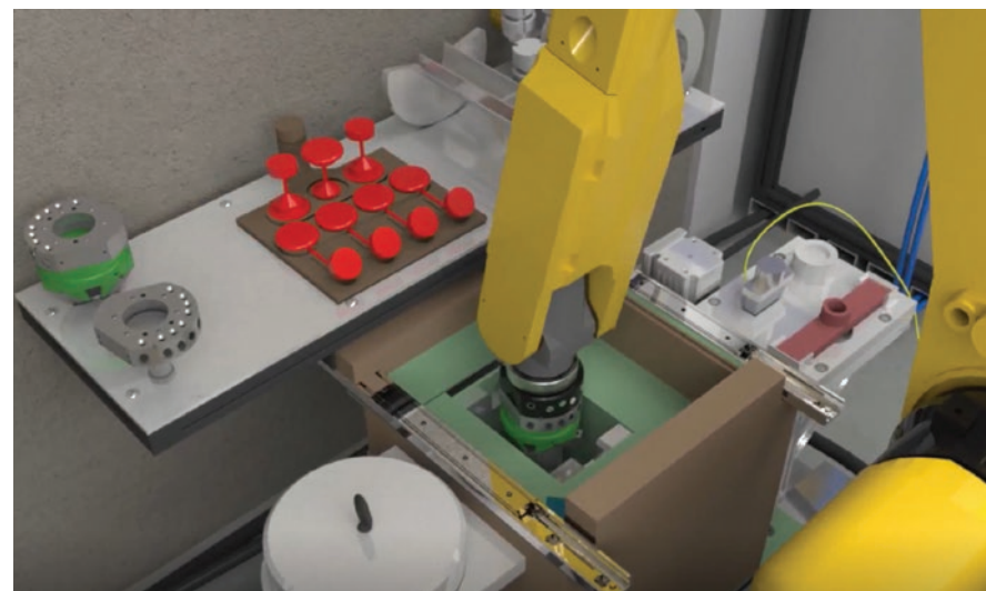
Illustration showing the Robot Packaging Skid inserting a target into a can (Kevin Hera, SRNL)
