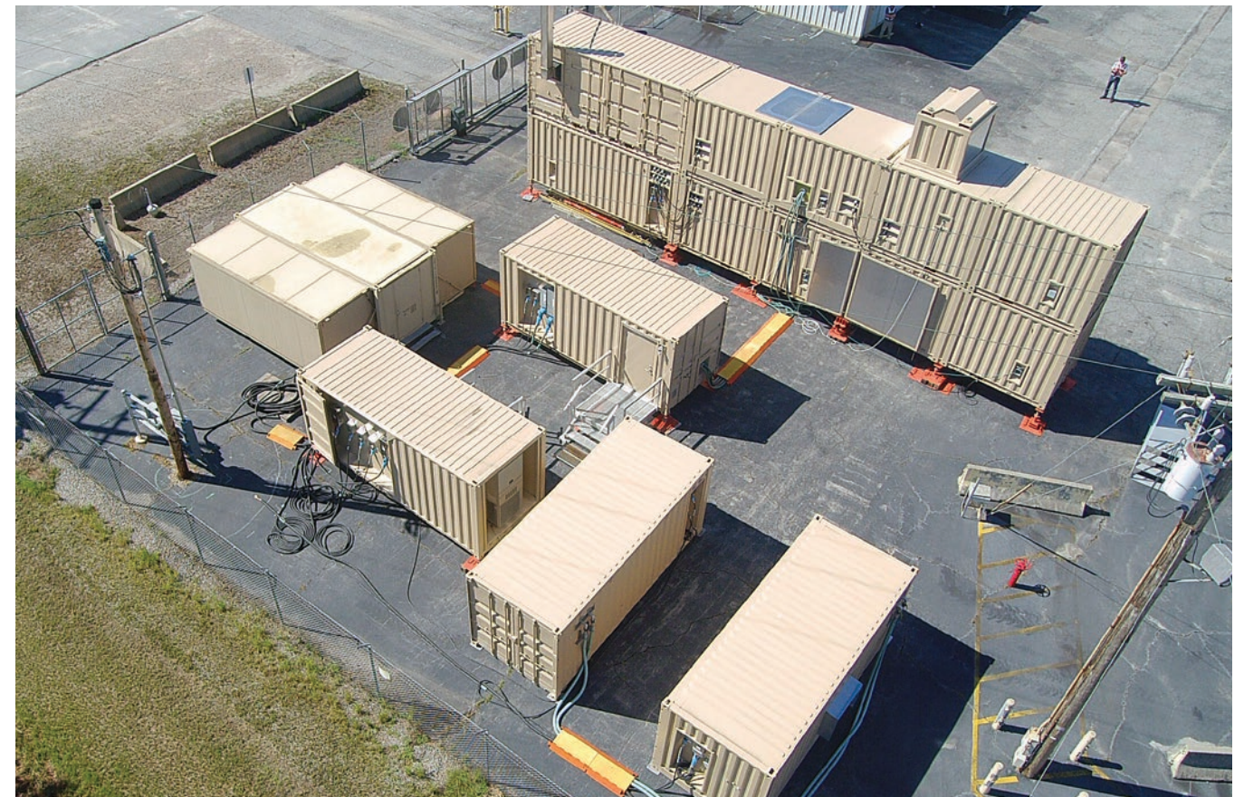
An aerial view of the Mobile Melt Consolidate. The system is made up of a collection of modules that work together to melt down spent nuclear fuel. (SRNL)
