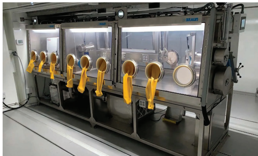
Glove boxes inside the Mobile Plutonium Facility (MPF) are used to do testing of nuclear materials on a small scale. (SRNL)
